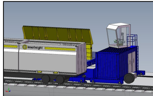
11 – Container layed down
